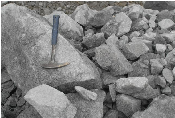
Photographs of recently blasted irregular and blocky shaped fragments of homogenous limestone. [Hammer 325 mm]
