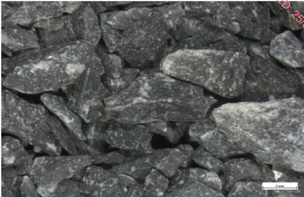
Retained 250 µm to 4 mm material from wet sieving. [Scale 2 mm]
