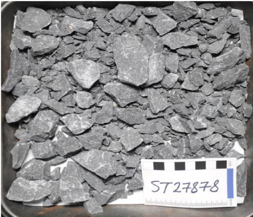
Retained >4 mm subsample on wet sieving. [Pan width 21 cm]
