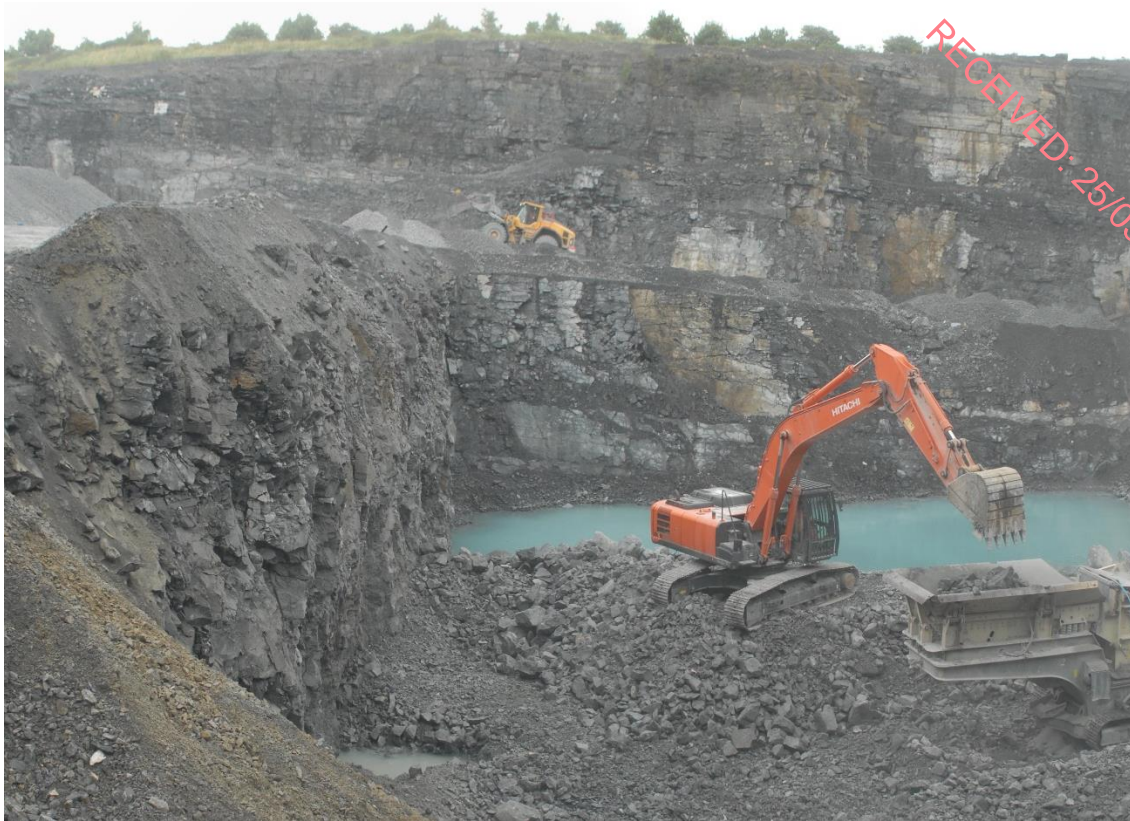
Photograph looking SE from IM 52035 13165 along active face with recently blasted material being processed.
