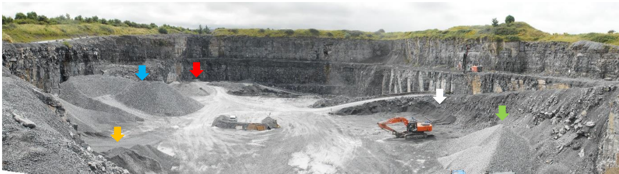
Panorama looking E to S to W from IM 52016 13283 with stockpiles of crusher run (red arrow), T0 Struc (blue arrow), T1 Struc (orange arrow), Cl. 505 (green arrow) and non-specified 3/4" down (white arrow). Small stockpile of T2 Perm obscured from view.
