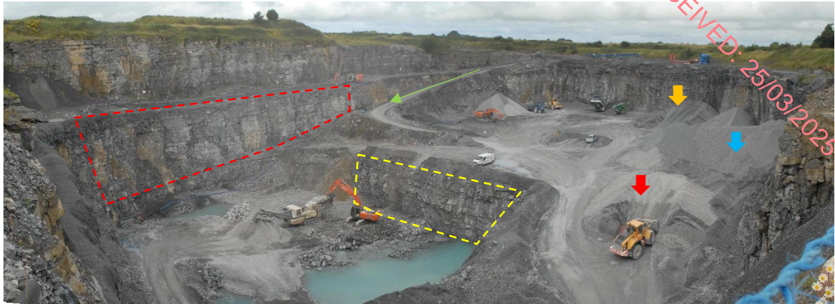
Panorama looking WNW to N from SW edge of quarry at IM 52157 13145 showing haul road to middle level (green arrow), active face (dashed yellow box), stockpiles of crusher run (red arrow), T0 Struc (blue arrow), T1 Struc (orange arrow). Small blast along ENE-WSW face (dashed red box) will enable haul road to be extended to quarry floor.
