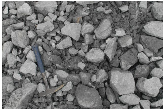
Photographs of recently blasted irregular and blocky shaped fragments of homogenous limestone. [Hammer 325 mm]
