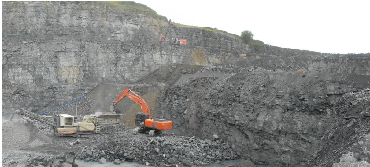
Active face on quarry floor looking SW to NW from IM 52108 13175. Rock in face largely obscured by dust. Brown (dolomitised) material behind excavator will be used to extend haul road.
